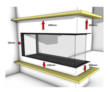
Ensure all clearances are met to any combustible or heat sensitive materials in front, above, to the side, or below the fireplace viewing area. Following these clearances, will allow the use of standard building materials, whether combustible or noncombustible. It is recommended to keep furnishings at least **1m** from the front of the fireplace.
