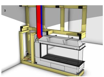
Install electrical, network connections, and gas supply.
