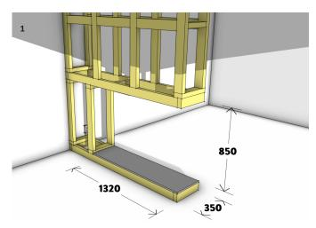
Build the chimney framework with consideration to flue pathways and meet the minimum fireplace opening requirements (1320mm W x 850mm H x 350mm D). Ensure a continuous base for the fireplace.
