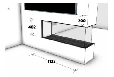
Attach wall linings to the framework and fireplace, maintaining a 3mm gap from the fireplace trim. Follow the provided wall lining cutout dimensions above for 20mm wall linings. Complete the project by adding additional finishes or fixtures.
