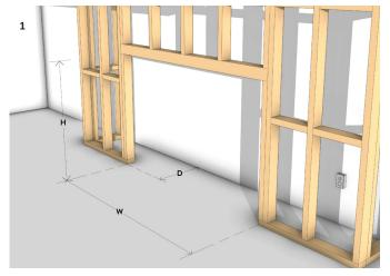
Build the chimney framework with consideration to flue pathways and meet the minimum fireplace opening requirement 1735 W x 1090 H x 465 D. Ensure a continuous base for the fireplace.
