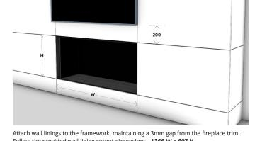
Attach wall linings to the framework, maintaining a 3mm gap from the fireplace trim. Follow the provided wall lining cutout dimensions - **1366 W x 607 H.**Complete the project by adding additional finishes or fixtures.
