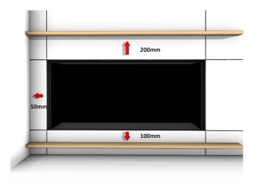
Ensure all clearances are met to any combustible or heat sensitive materials in front, above, to the side, or below the fireplace viewing area. Following these clearances, will allow the use of standard building materials, whether combustible or noncombustible. To reduce these clearances, use non-combustible materials.
