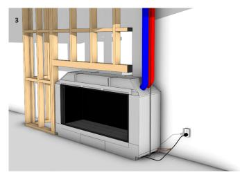
Connect flue pipes to the fireplace and create the flue pathway to the terminal.
