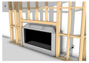
Install the appliance into the preformed cavity opening and secure it to the base. Ensure the fireplace is flush with the framework. Provide mains power connection and an accessible isolation switch. Install electrical, network connections, and gas supply.
