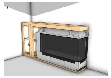
Install the appliance into the KWU Framework and secure it to the base. Ensure the fireplace is flush with the framework. Provide mains power connection and an accessible isolation switch. Install electrical, network connections, and gas supply.
