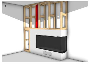
Connect flue pipes to the fireplace and create the flue pathway to the terminal. Connect Powerflue electrical cable at both ends. Fit KWU last side and front panels onto framework. Build the remainder of the framework where required.
