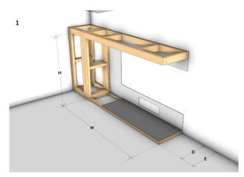
Build the KS1460 KWU framework and fit the rear panel - 1850 W x 1200 H x 453 D. Surrounding framework and KWU must be 466mm (E) off the rear wall. Consider the flue pathway. Ensure a continuous base for the fireplace.
