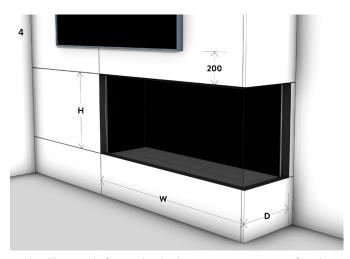
Attach wall linings to the framework and and KWU, maintaining a 3mm gap from the fireplace trim. Follow the wall lining cutout dimensions -  $1408 \text{ W} \times 607 \text{ H} \times 434 \text{ D}$ . Complete the project by adding additional finishes or fixtures.
